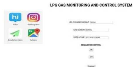
Figure: 9 Web page-based app for monitoring and control
